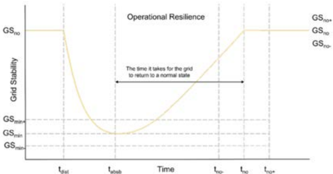
Figure 3: Operational Resilience Represented Graphically with respect to time to return to normal
